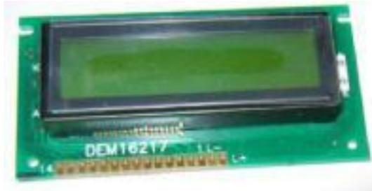
Figure 1: A typical LCD module
