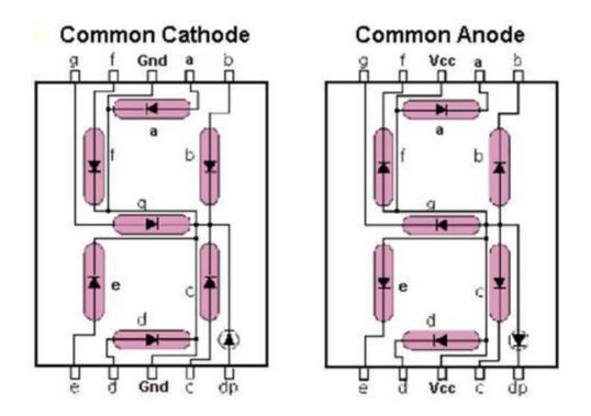
Interfacing a Seven-Segment display is independent of the type of the module, whether it is common anode or common cathode, only the logic level sent to the display differs. Finally, since the display is basically LEDs, current limiting resistors are used for each segment.
