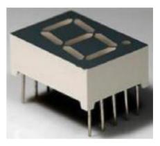
common cathode display. To switch a LED on in a common cathode configuration, you have to send logic high to the segment pin. Conversely, to switch a LED on in a common anode configuration, you have to send logic low to the segment pin.
