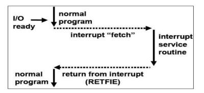
Interrupts can be thought of as *hardware-initiated subroutine calls*. Usually, interrupts are generated by I/O devices such as timers or external devices.
