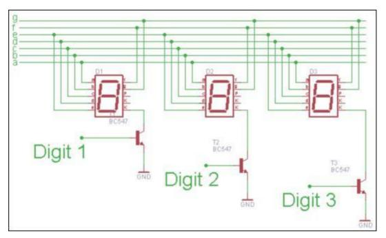
Figure 3: 7-segment multiplexing of 3 digits
