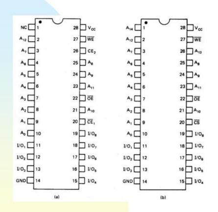
4364 and 43256A pin layouts are designed for compatibility 4364 pin configuration (Fig a)
