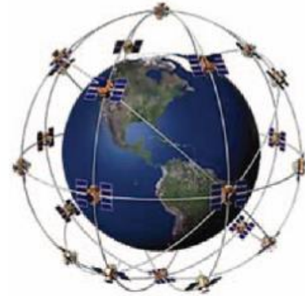
Figure TF5-2: GPS nominal satellite constellation. Four satellites in each plane, 20,200 km altitudes, 55° inclination.
