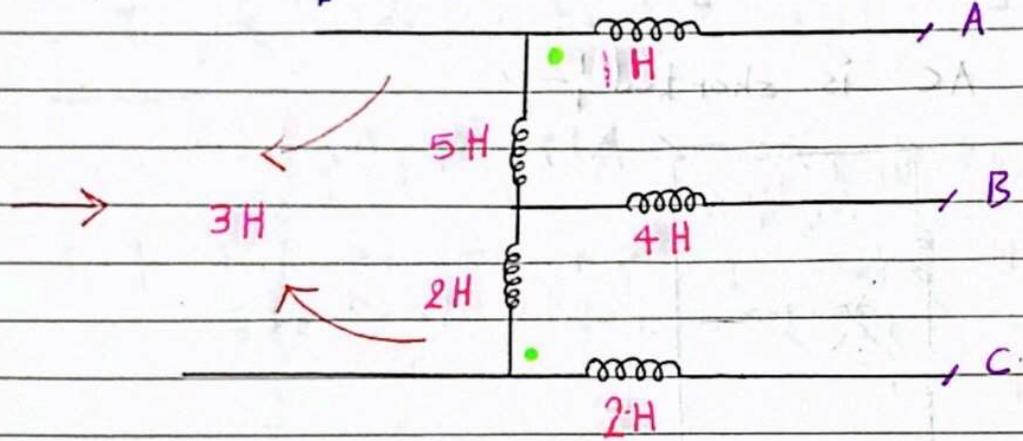
① When there are no connection between A and B and C :-
