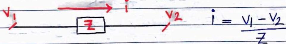
⊙ 1- By using Nodal analysis و Find  $[v_1 / i_1 / i_2]$ .
