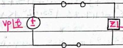
So 1 - This demonstrates [single phase system] with [two wires system].
