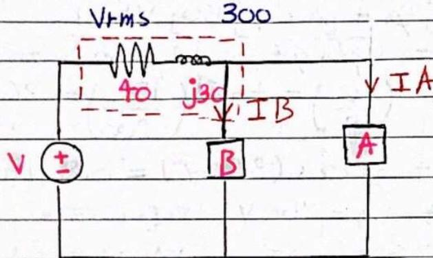
Q1 - Three loads are connected in parallel across the  $500 \angle 0^\circ \text{ V}_{\text{rms}}$  source shown below:-
