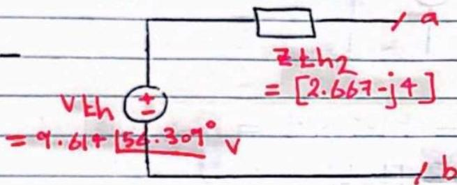
⊗ :- obtain the equivalent circuit at terminals (a-b) :-
