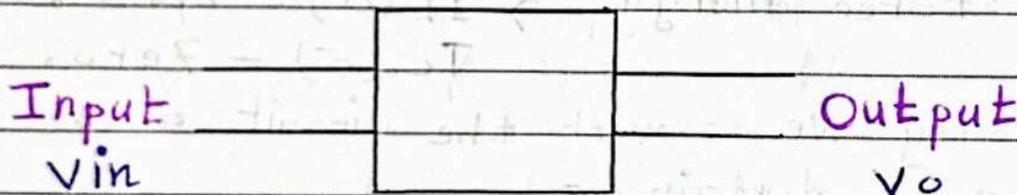
$$\text{Transfer Function (H)} = \frac{V_o}{V_{in}}$$
