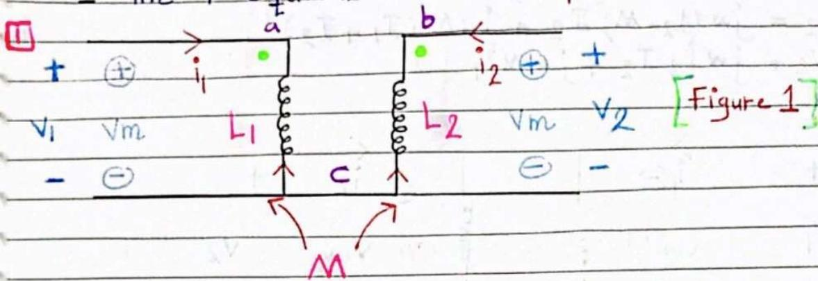
sol:- The T equivalent circuit for the linear transformation above :-
