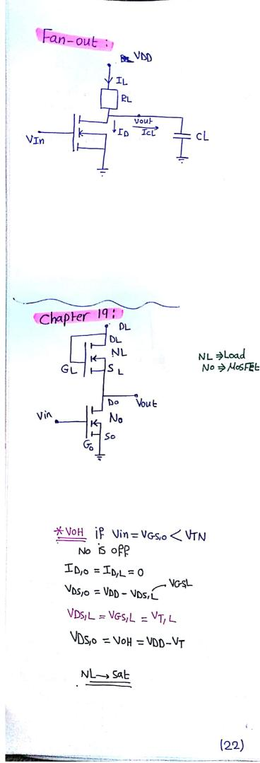
\* when I/P(Low) ( high high Low VGS < VTN NMOS OFP  $I_L = I_{CL} = C_L \frac{dV_C}{dt}$ ("Low -high) \* When I/p (high) NMOS pull down , Linear Idis = -Icl  $= -CL \frac{dVC}{dL} = -(I_L - I_D)$ IcL = IL - ID  $I_{CL} = C_L \frac{dV}{dL}$ Idis = - CL dv \* VDS,L = VGS,L because ,GL are Connected \*VDSL(Sat) = VGSL - VTLVDS L VDSL >VDSL(Sat) NMOS SAL IDL = IDO \* VOUF = VDSO = VDD- VDSIL VDS, L = VDD - VDSO = VGS, L
