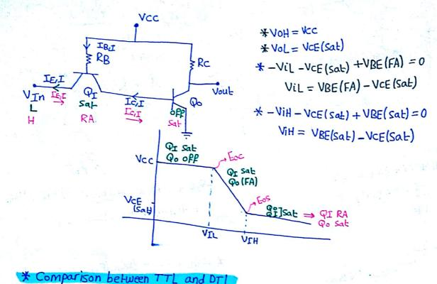
① DI, DL in DTL is replaced by QI
