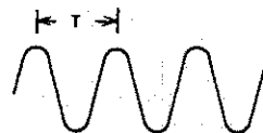
Figure 1-11 A wave having period T seconds. The corresponding frequency is f = 1/T .
