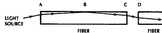
Figure 3-19 Reflecting surfaces in a fiber system. Light rays are reflected at the input (A), at the core interface (B), and at the boundaries of an air gap formed at a connector or splice (C or D).
