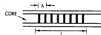
Figure 9-45 Fiber Bragg grating. The core's refractive index varies periodically along the axis.
