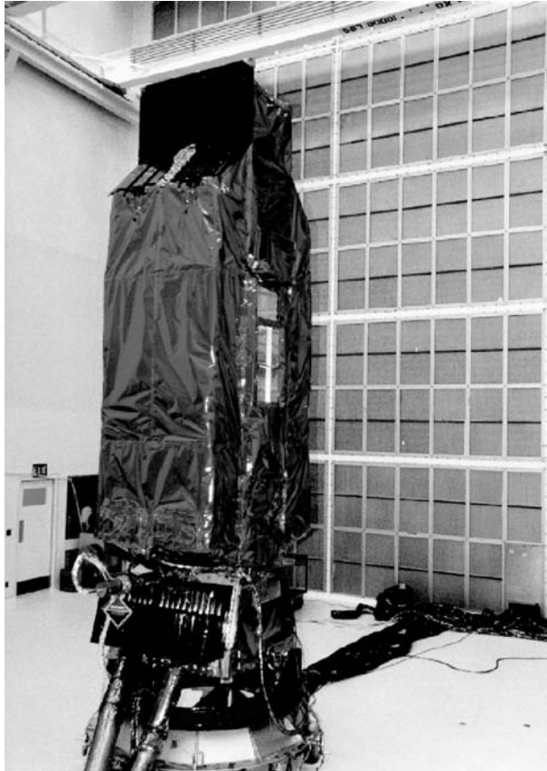
Figure 4.10 Thermal blanketing on FUSE satellite (Courtesy: NASA/FUSE Project at JHU)
