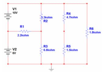
3.provide the DMM to measured the voltage& then determine the polarity of the voltage across the resistance as in the **sheet** (where the red probe in the +ve pole & the black in the ve), then measured the voltage across each resistance & record the values in the table.
