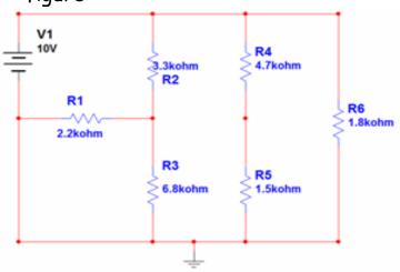
provide the DMM to measured the voltage& then determine the polarity of the voltage across the resistance as in the <u>sheet</u> (where the red probe in the +ve pole & the black in the -ve), then measured the voltage across each resistance & record the values in the table.
