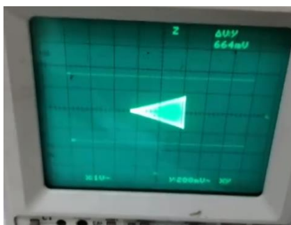
trapezoidal pattern to get 100% modulation.
