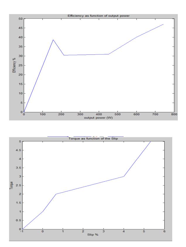
The difference is due to friction with air, so when the torque is zero, we the motor will rotate at faster speed (to overcome the friction of air) than the synchronous speed and the motor becomes a generator.
