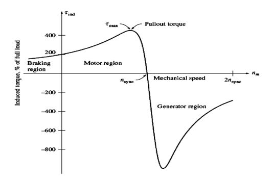
Note : nm = (1-s) \* n synch, so this curve also represents the torque as a function of the slip with a shift and reflection about the torque axis.
