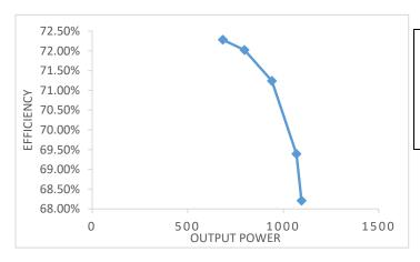
We can note from the figure that the output power is inversely proportional to efficiency because the increase in power comes from the increase in the current, and then the losses will increase.
