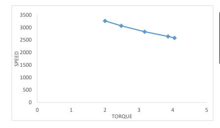
We can note from the figure that the torque is inversely proportional to speed, as the greater torque, the lower the speed
