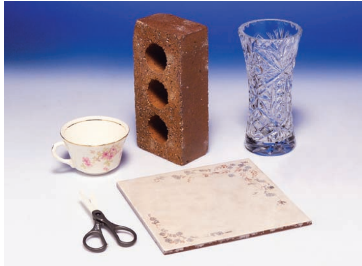
Figure 1.9 Common objects that are made of ceramic materials: scissors, a china teacup, a building brick, a floor tile, and a glass vase.
